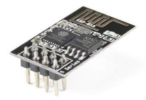
Designed as a standalone system-in-a-chp, this Wi-Fi module includes a TCP/IP protocol stack, 4MB of reminiscence, and a multitude of additional hardware (regulators, amplifiers, and so forth.). This will allow any microcontroller, consisting of an Arduino board, to access your Wi-Fi community connected in the project.
