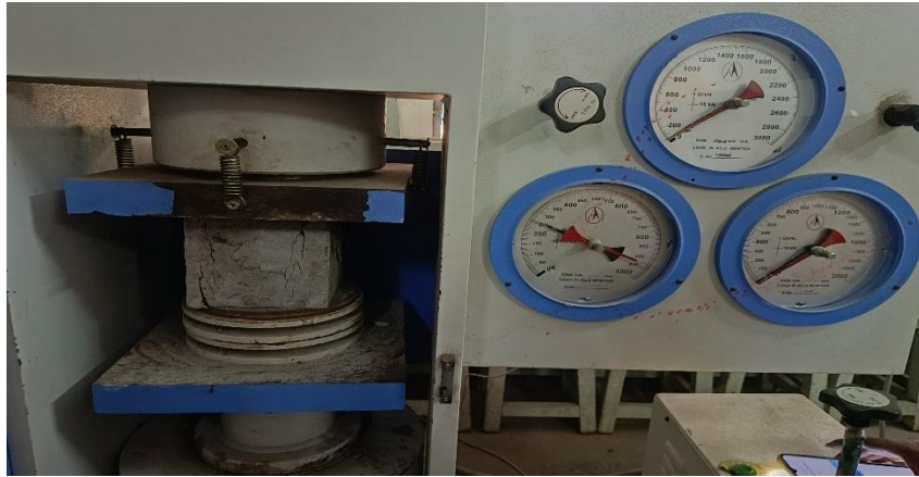
Fig3: Compressive strength test
