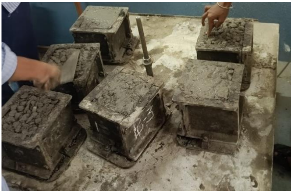
Fig1: Casting of cubes
