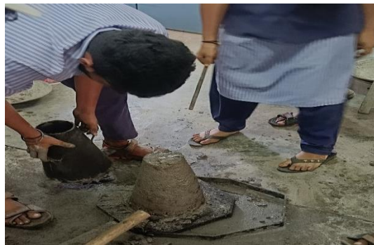
Fig4: Slump cone test
