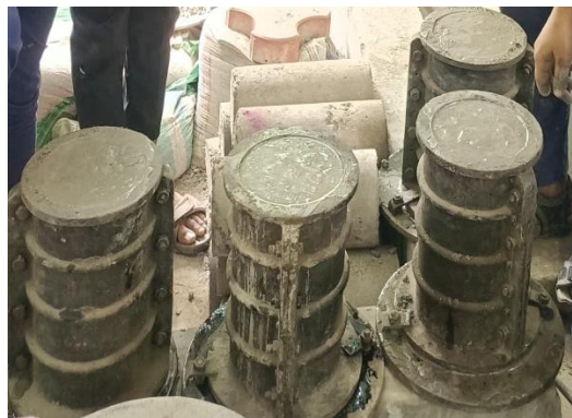
Fig2: Casting of cylinders
