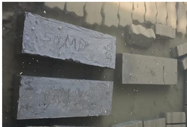
Fig no: 23 Curing of Foam Blocks
