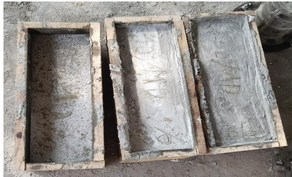
Fig no: 21 Casting of Foam Blocks
