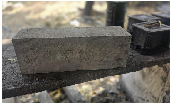
Fig no: 22 Foam Block after Demoulding
