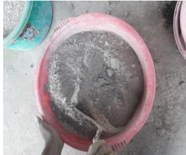
Fig no: 16 Dry mix of cement, fly ash and Slaked lime
