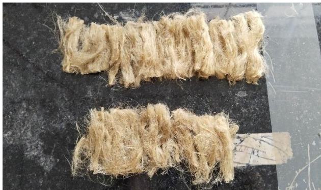
Fig no: 13 (a),(b) To cast the blocks, kenaf fiber was chopped into 50 mm (5cm) pieces.
