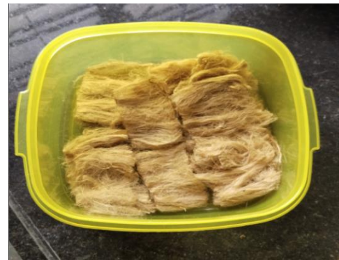
Fig no: 13 (a),(b) To cast the blocks, kenaf fiber was chopped into 50 mm (5cm) pieces.
