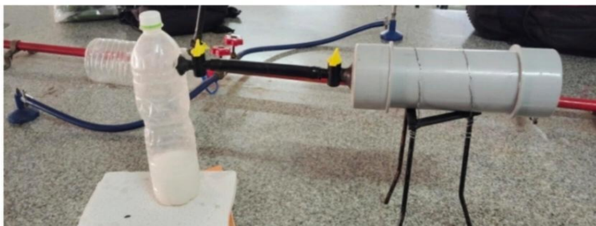
Fig 2.4 Experimental setup for CO 2 absorption
