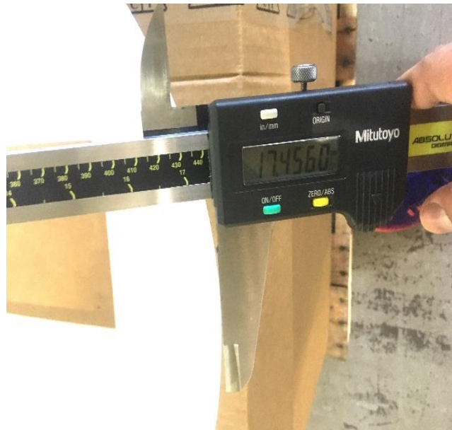
Figure 3. Vertically in-spec part using the cooling fixture
