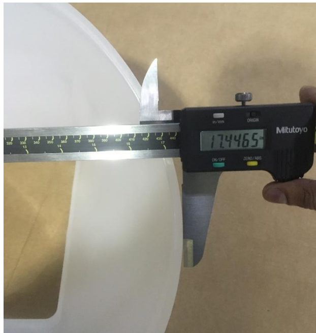
Figure 4. Horizontally in-spec part showing OD roundness improvement
