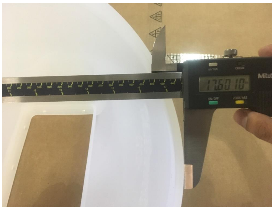
Figure 1 : the parts shrinks one side more than the other, ending up with oval shape
